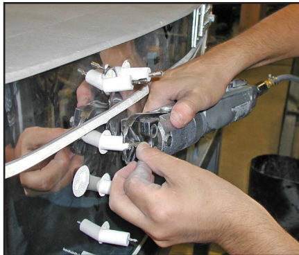
Crimping high temp connector on pigtail
