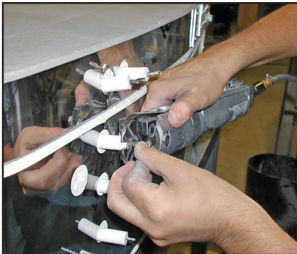
Crimping high temp connector on pigtail
