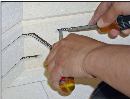
Inserting element into brick groove
