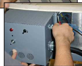
Removing screws attaching electrical box to kiln and gently pulling box away
