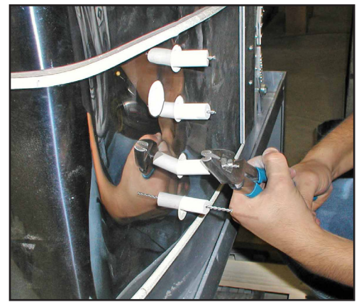
Cutting pigtail to connect to high temp connectors
