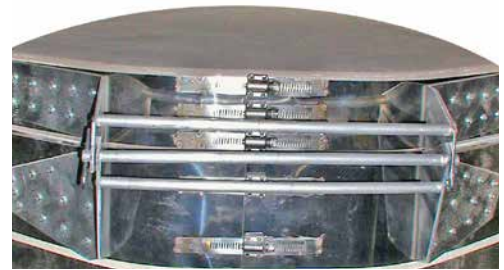
Repositioning Lid when Thermal Expansion Occurs
