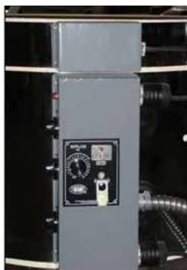
Detach screws from kiln sitter plate
