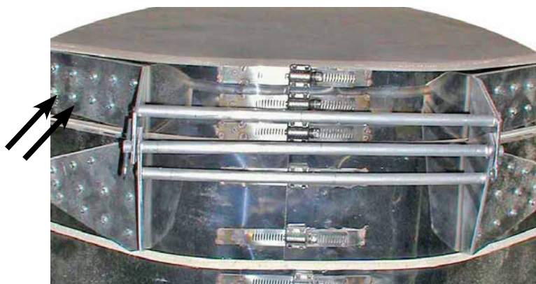
Repositioning Lid when Thermal Expansion Occurs
