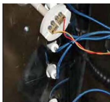
Insert thermocouple through kiln sitter hole
