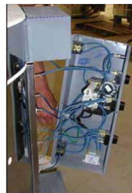
Remove wires from back of kiln sitter terminal block
