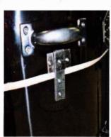
Step 10 With the lid opened, attach safety wire first and then attach spring by pulling up on the spring.
