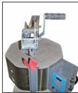
Hand Crank to lift firing chamber
