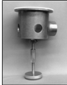
Collector cup with gasket, adjustable height foot, stud, coupling and wing nut
