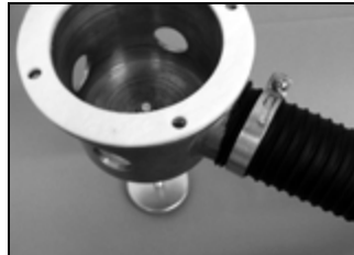
High temperature black flex hose attached to collector cup
