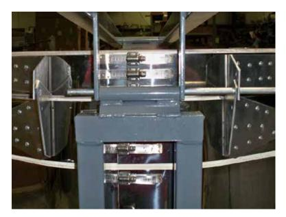
Remove cotter pin from one side of the stiffening rod. Slide stiffening rod out of holes. Lid Lift arm will be unattached in back.
