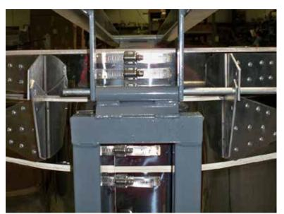
Place Lid Lift arm on top of the kiln lid. Position holes in Lid Lift arm and frame. Insert stiffening rod through holes and attach cotter pin.
