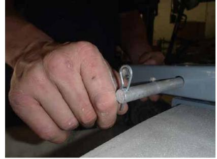
Removal of Firing Chamber from Frame
