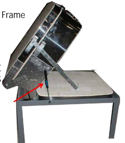
Remove bolts on back of the kiln with the kiln chamber closed. The kiln floor will remain attached to the kiln frame.
