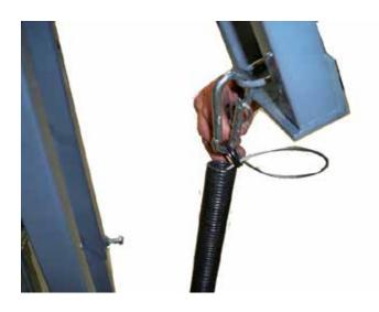
Remove Lid Lift Arm. This is a 2 person job. Have 1 individual lift the kiln lid straight up and the other person remove the ring lock from lid arm. The individual lifting the lid will feel the weight of the kiln lid once the spring is no longer attached. Slowly lower lid to the closed position.
