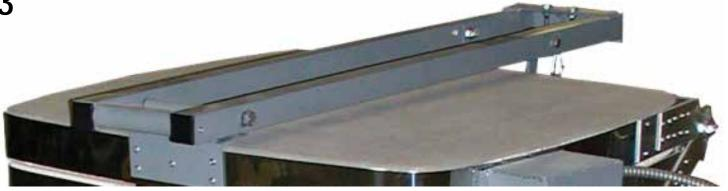
Remove cotter pin from one side of the bolt on the front of Lid Lift arm. Slide bolt out of holes. Lid Lift arm will be unattached in front and can be removed from the kiln.
