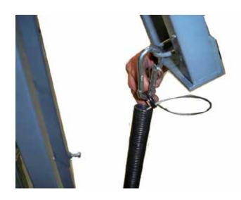
Have 1 individual lift the kiln lid straight up and the other person attach the spring with ring lock to lid arm. The kiln will be assembled and ready to fire.
