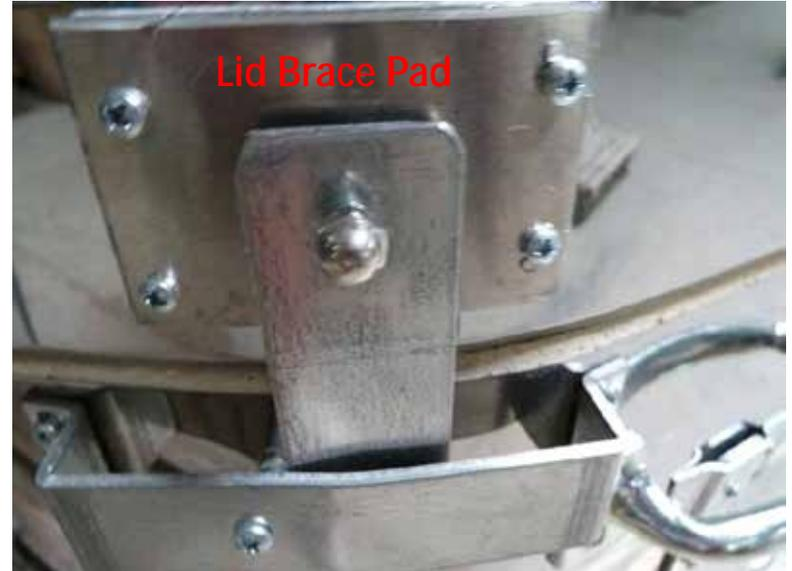
Lid Brace Arm – angle cut faces back of kiln. Unscrew nut on lid brace pad, insert the top of the lid brace arm through the body brace and through the lid brace pad. Insert hole in top of arm onto bolt and attach nut.
