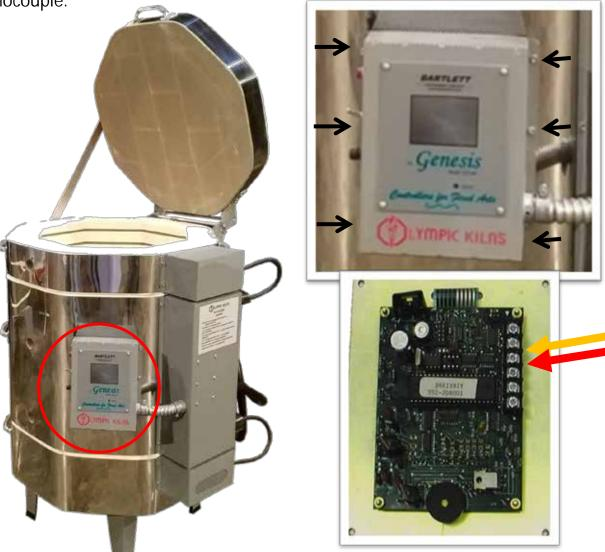
Remove the screws on both sides of the electrical box housing the electronic controller. Strip the thermocouple's yellow and red wires 3/8 of an inch. Disconnect defective thermocouple and insert new thermocouple with the fiber (if needed) through the opening in the kiln brick. Set the thermocouple approximately 1" inside the kiln firing chamber. Attach thermocouple's yellow wire to the positive connection on the electronic board and the red wire to the negative connection.
